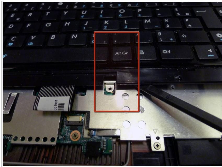
ⓘ At this step, the keyboard is still maintained with double-sided tape between the keyboard underside and the metallic PCB protector.
