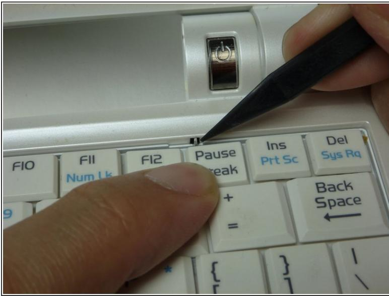
**⚠ Caution** Follow this step to detach the upper portion of the keyboard, but do not remove it from the laptop. Damage to the keyboard's ribbon cable may result if improperly executed.
