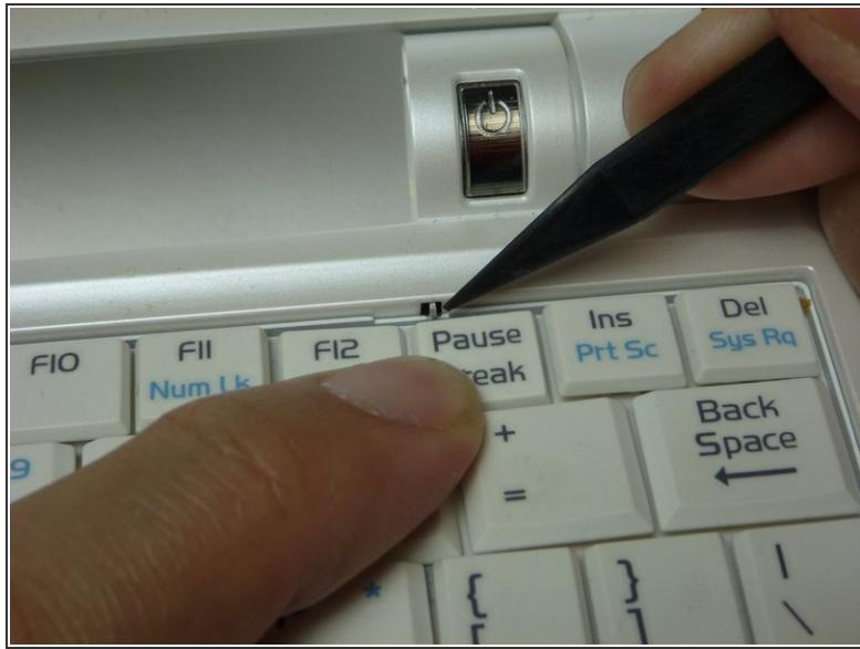
**⚠ Caution** Follow this step to detach the upper portion of the keyboard, but do not remove it from the laptop. Damage to the keyboard's ribbon cable may result if improperly executed.
