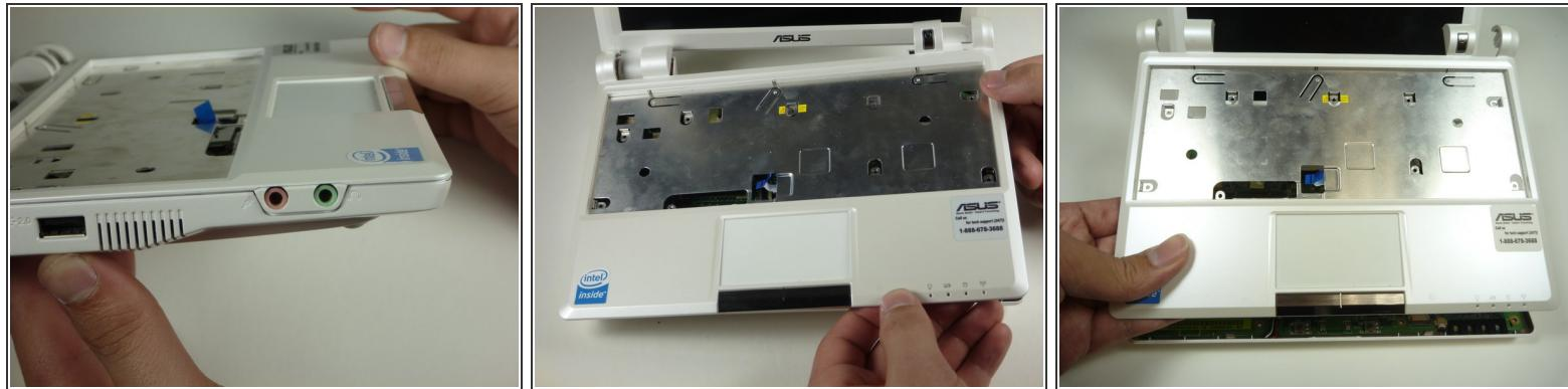
**⚠ Caution:** You will need to clear the audio and microphone jacks by lifting the right half and then moving the cover to the left (as shown in the second picture) to prevent damaging the cover.
