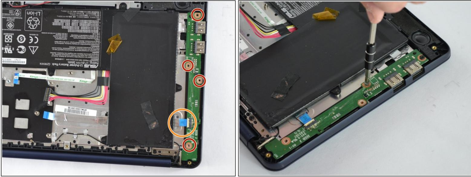
*(i)* The USB ports are located on the strip that looks like the motherboard on the left side of the laptop next to the battery.
