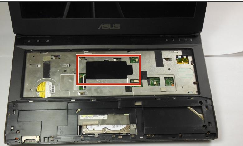
*(i)* If you want to add additional RAM, more ports can be found underneath the black plastic flap on the top side of the laptop, just under the keyboard. These ports behave the same way as the ones on the backside of the computer.
