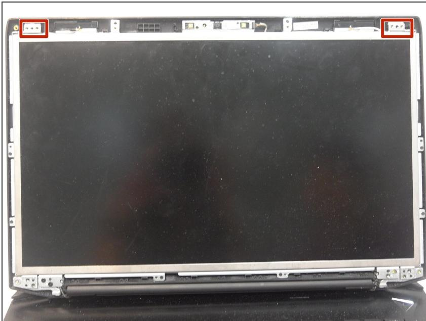
With the screws removed, the metal bracket surrounding the screen will feel loose.
