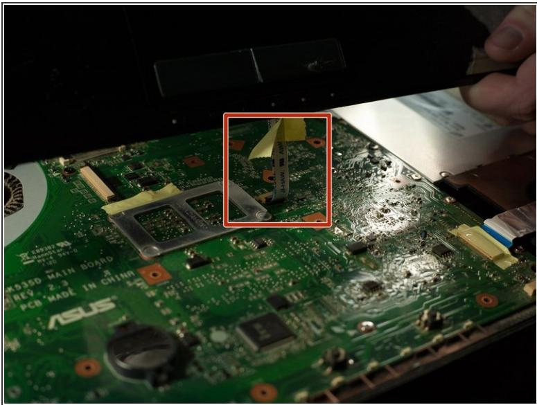
**⚠** There is a ribbon connector that is connecting the two halves of the laptop. So when opening the two plastic pieces be careful not to damage the cable.
