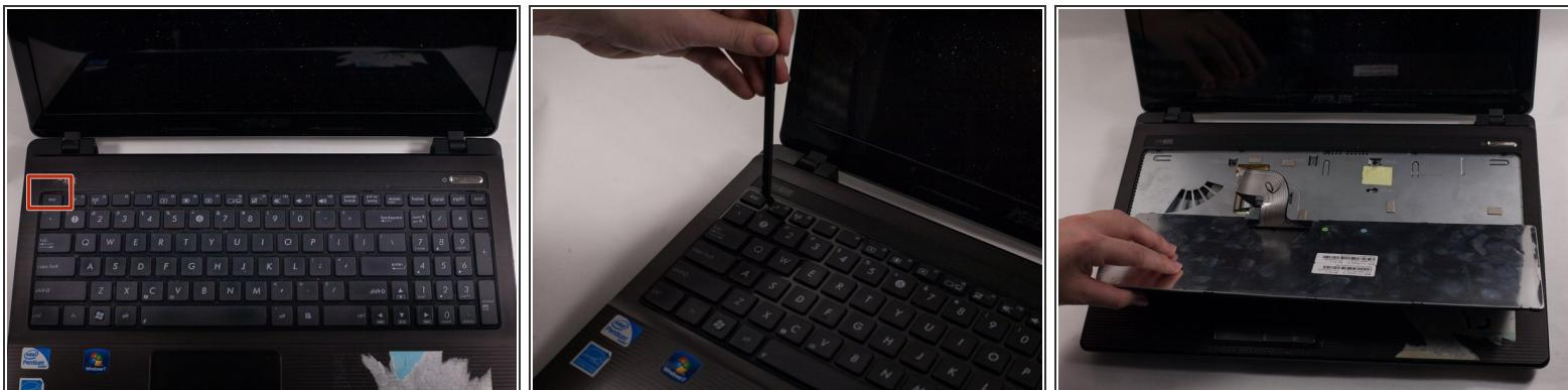
! There is a ribbon connector underneath the keyboard. When lifting up the keyboard be gentle and carefully lift it up.
