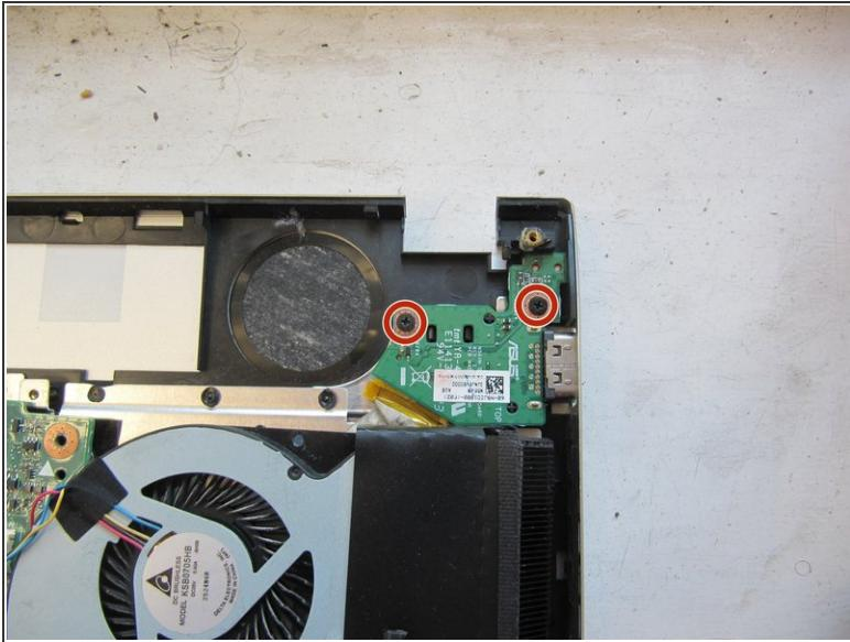
*(i)* This component is attached by a cable to the lower side of the motherboard therefore it is advised to remove it.
