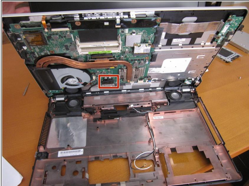
*i* The motherboard is still connected to the bottom case by several cables, so don't try to remove it entirely just yet.
