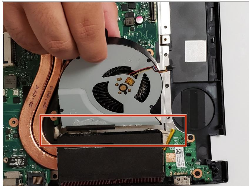
**⚠** The fan is glued to the black box that it is inside of. When pulling the fan out, you may experience a small amount of tearing of the black box.
