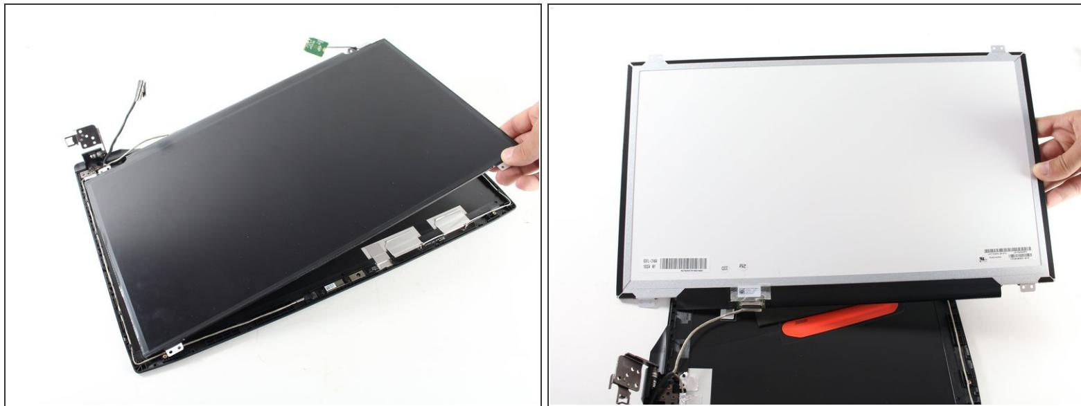
**⚠** When lifting, be sure to not strain the wires on the left side of the photo, as that could lead to a malfunction in the wires.
