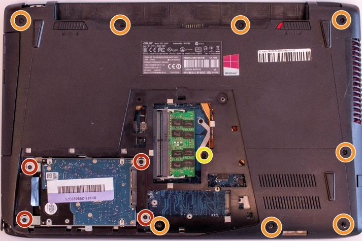
**i** The following screws will be removed using the Phillips #1 screwdriver.
