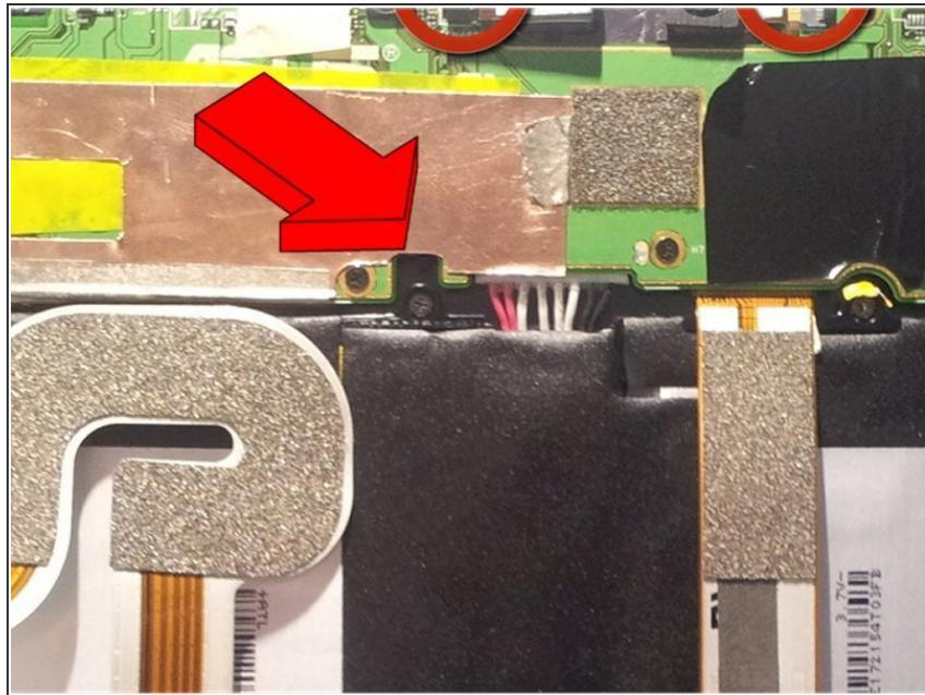
*ⓘ* There is an internal power switch next to the battery connector, that will kill power to the entire device while you're working on it.
