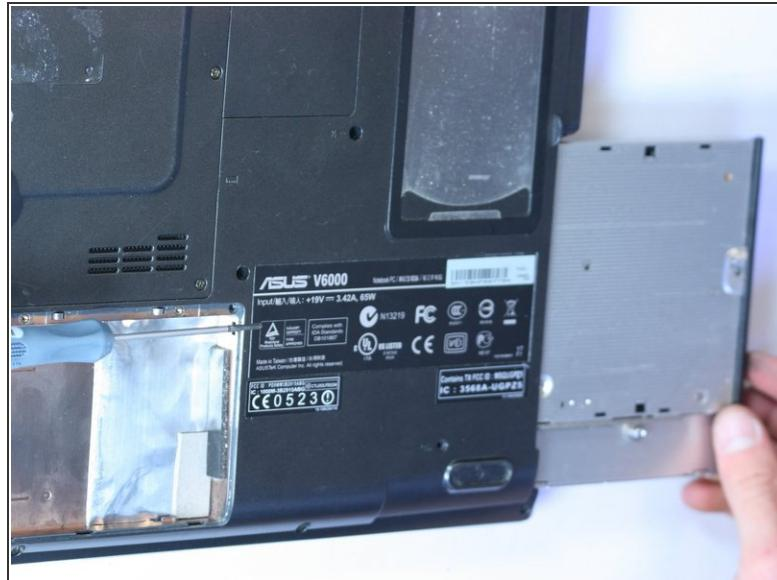
⚠ First, remove the highlighted screw (bottom right corner in the picture.)
