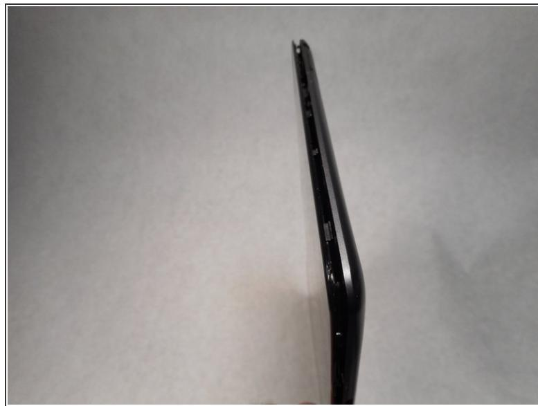
*(i)* Use the plastic opening tool to help detach the screen from the back panel.
