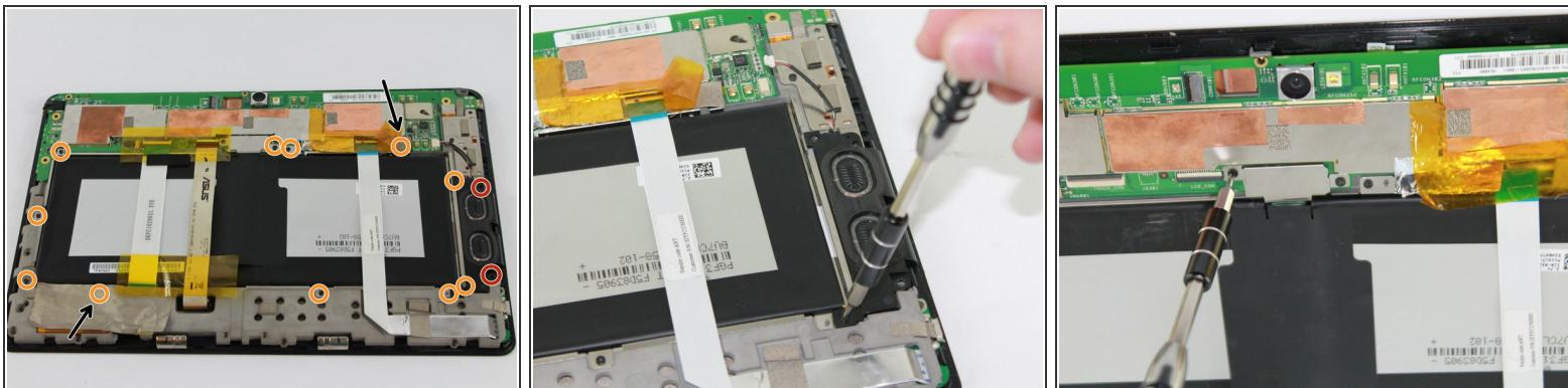
***(i)*** The Philips #00 Screwdriver listed in the recommended tools will fit all the screws.
