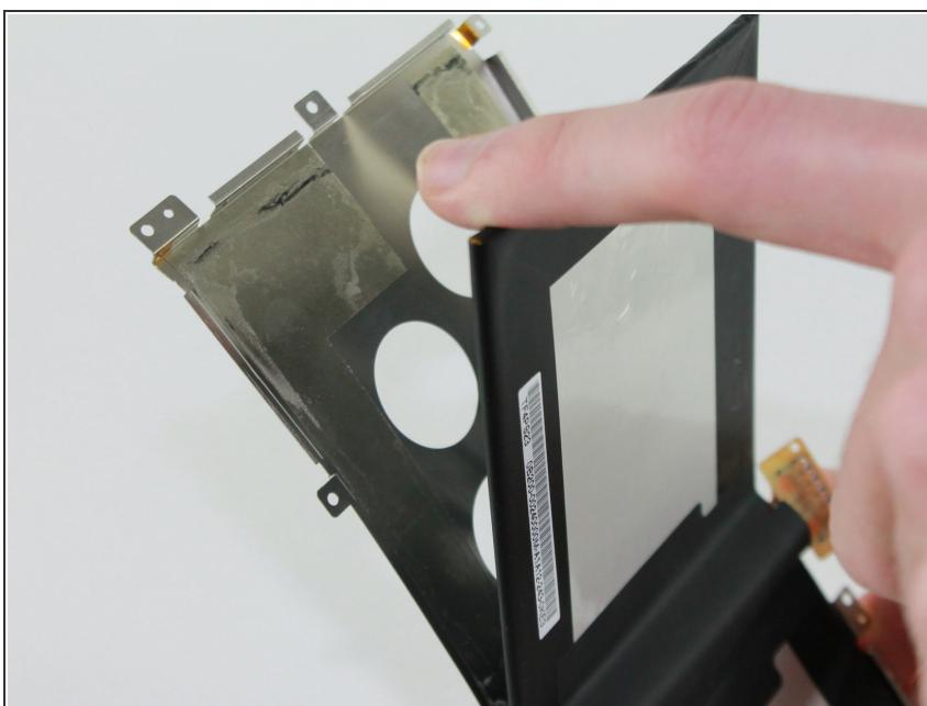
**!** The battery is secured to the tray by a strong adhesive. Take care not to bend the tray when removing the battery.
