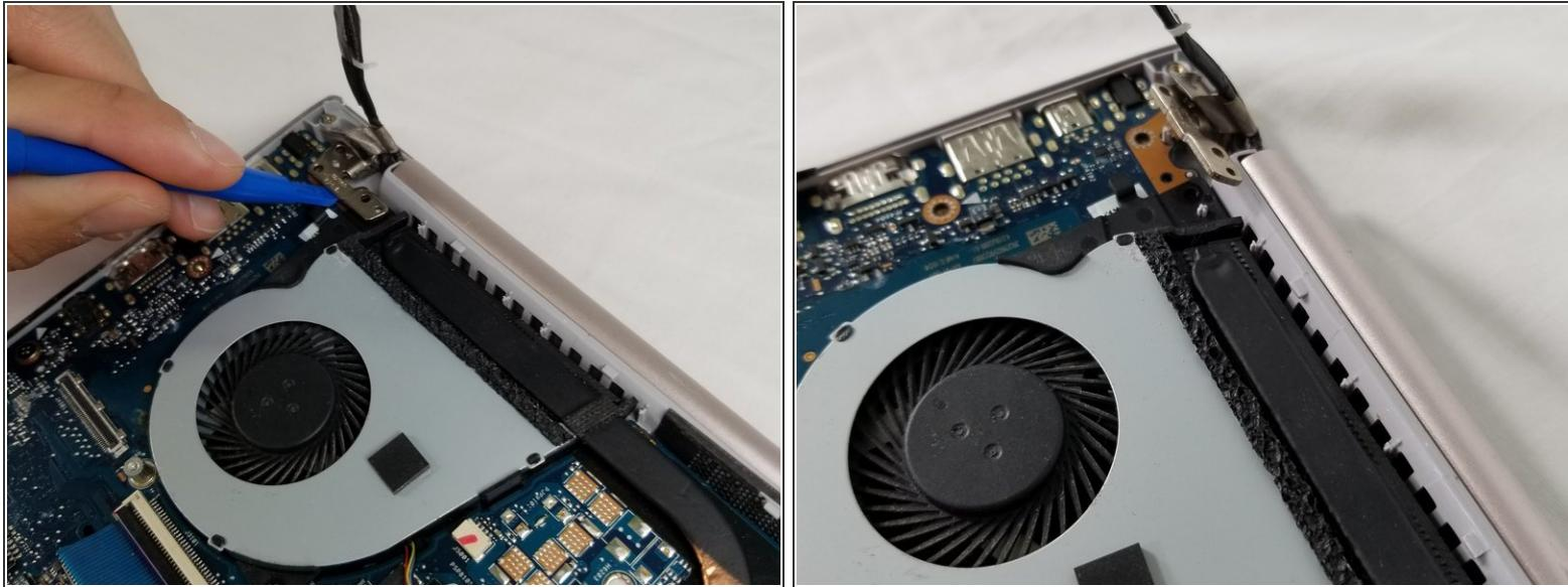
ⓘ Lift the bottom of the laptop up slightly in order to unhinge the laptop.
