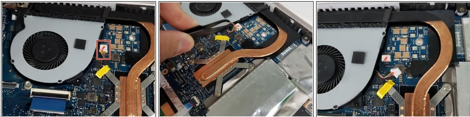
● Using tweezers, disconnect the cable connector from the motherboard fan.
