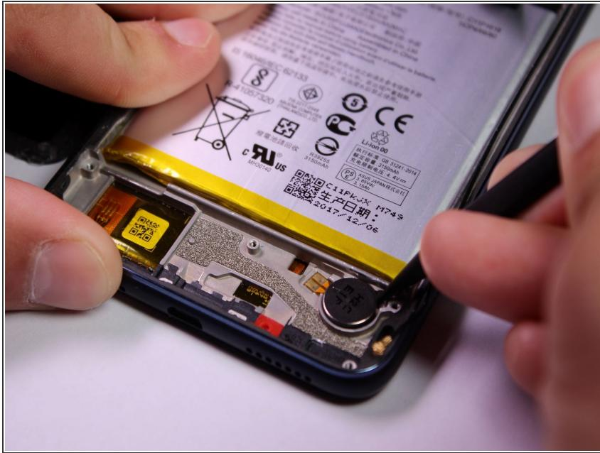
*(i)* The vibration motor is the circular metallic piece located on the bottom right of the phone.
