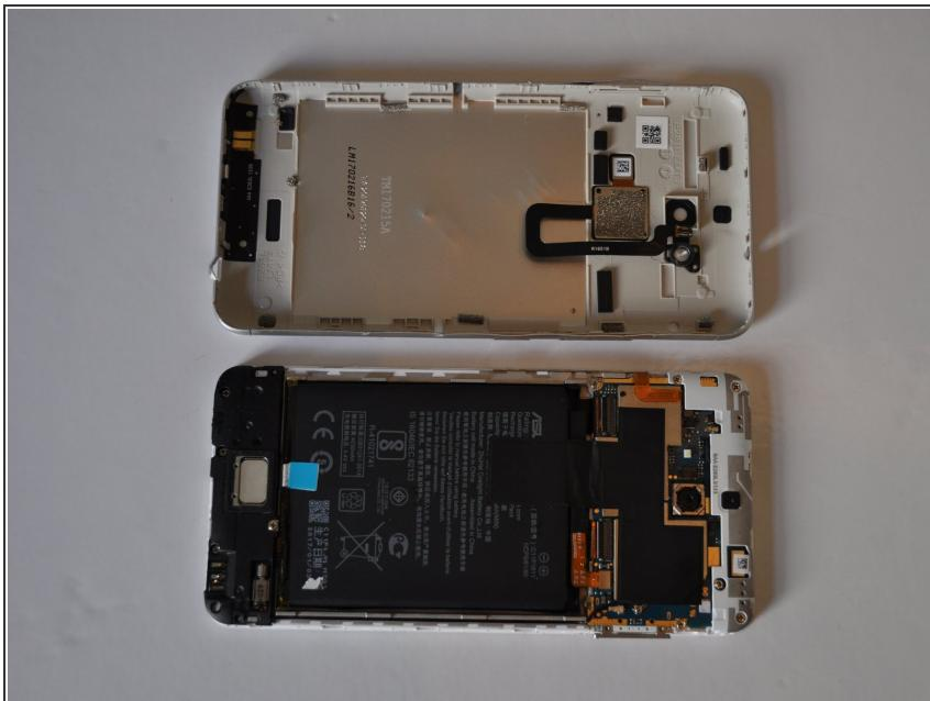
Once the original cover has been removed, apply the new cover to the back of the phone with careful pressure.
