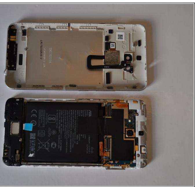
Once the original cover has been removed, apply the new cover to the back of the phone with careful pressure.
