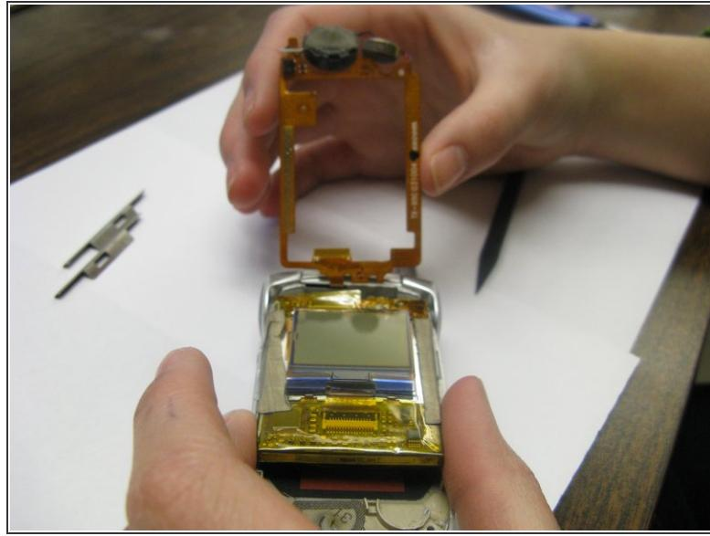
⚠ The copper frame is attached to the phone at the hinge. Do not tear the frame.
