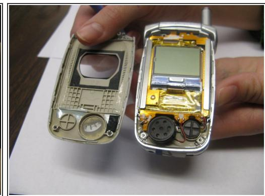
! The small electronic components inside the phone are fragile; take care not to damage them when completing this step.
