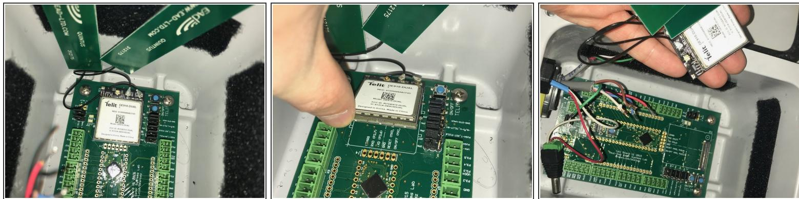
⚠ Pull the module from the bottom; pulling the module in a different way may damage it
