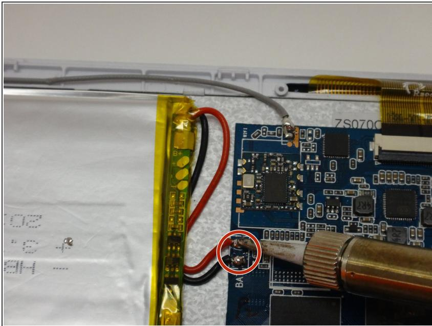
⚠ A soldering iron can reach 600° F, which will cause serious burns. Learn how to solder properly [here](#). Using tweezers to hold the wires will reduce the risk of burns.
