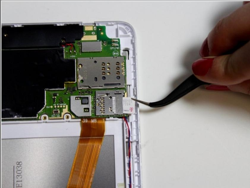
*(i)* You should be able to remove the SIM card without removing the back cover. The cover has been removed to more clearly show the SIM card.
