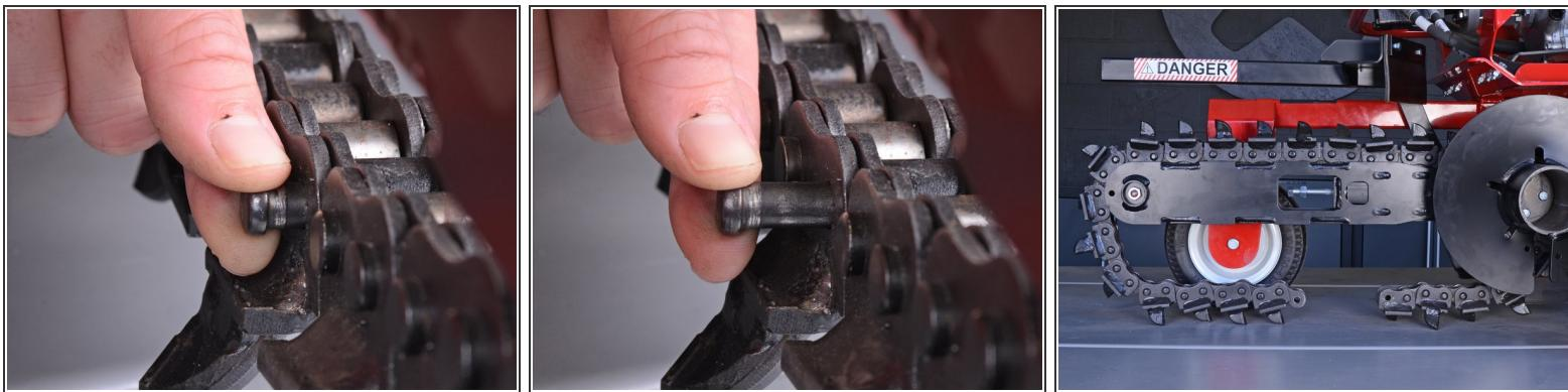
**⚠** The chain is very heavy and will drop off the boom as soon as the pin is removed from the master link. Make sure your hands are out of the way and nothing fragile is underneath the chain before you remove the pin.
