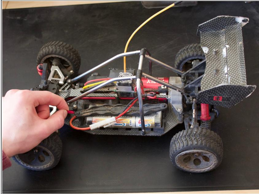
**i** TIP: Since this work has to be done more often, it is recommended to provide the cotter pins with some insulating tape so that they can be removed without tools
