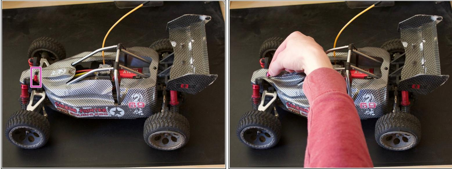
*(i)* TIP: if you remove the cladding more often (for example, for thorough cleaning), it may be helpful to provide the splints with some insulating tape, so the use of tools is unnecessary
