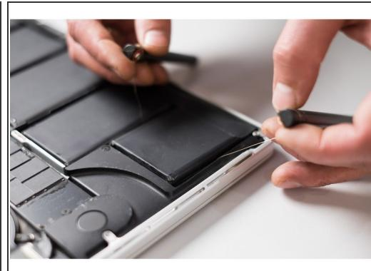
⚠ There is risk to damage the battery! (Do not use ANY metal tools - puncturing the battery can cause fire and possibly leak battery gel!)
