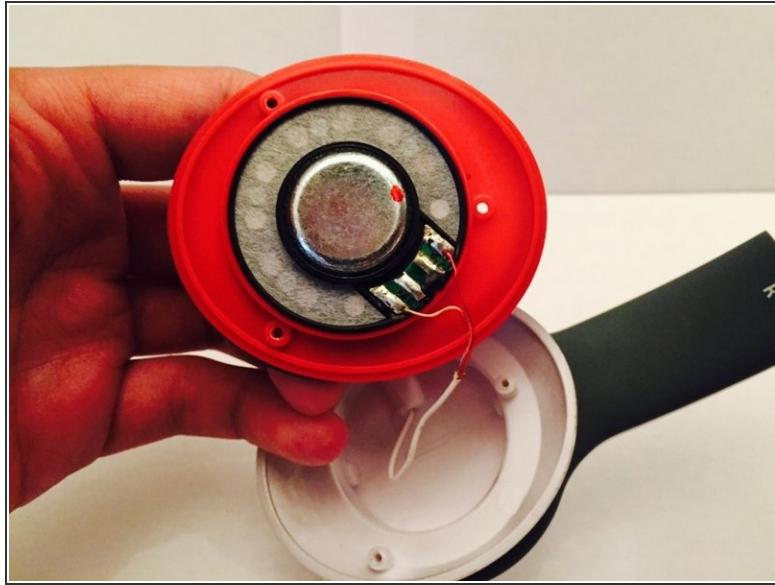
⚠ Using safety gloves, desolder the two wires of the speaker.
