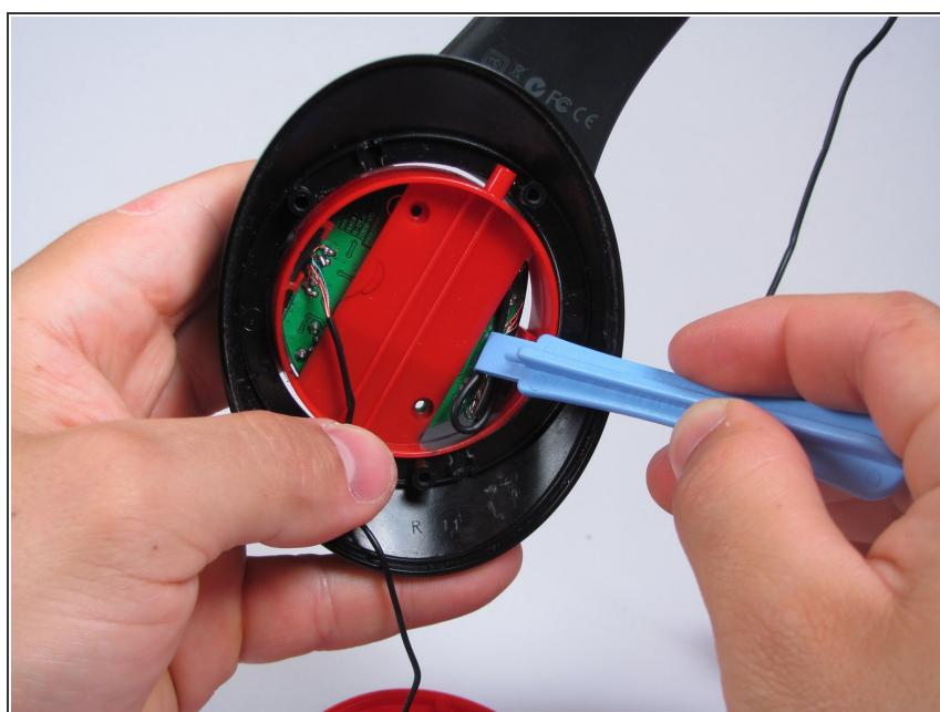
*i* Sometimes the motherboard will just fall out of its housing. If it doesn't, use a plastic opening tool to gently pry or push out.
