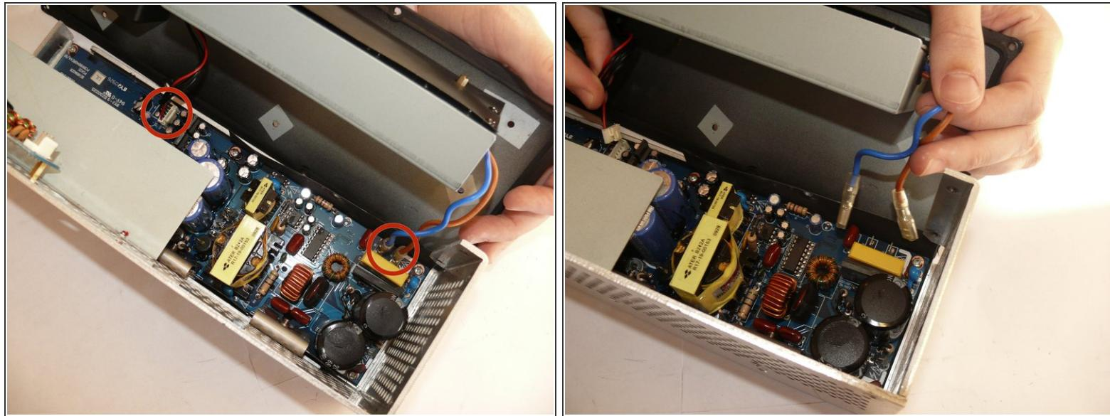
**⚠ Caution:** The circuit board contains many capacitors that could cause serious injury if touched. If possible, use a [capacitor discharge probe](#) to safely rid the capacitors of dangerous charges.
