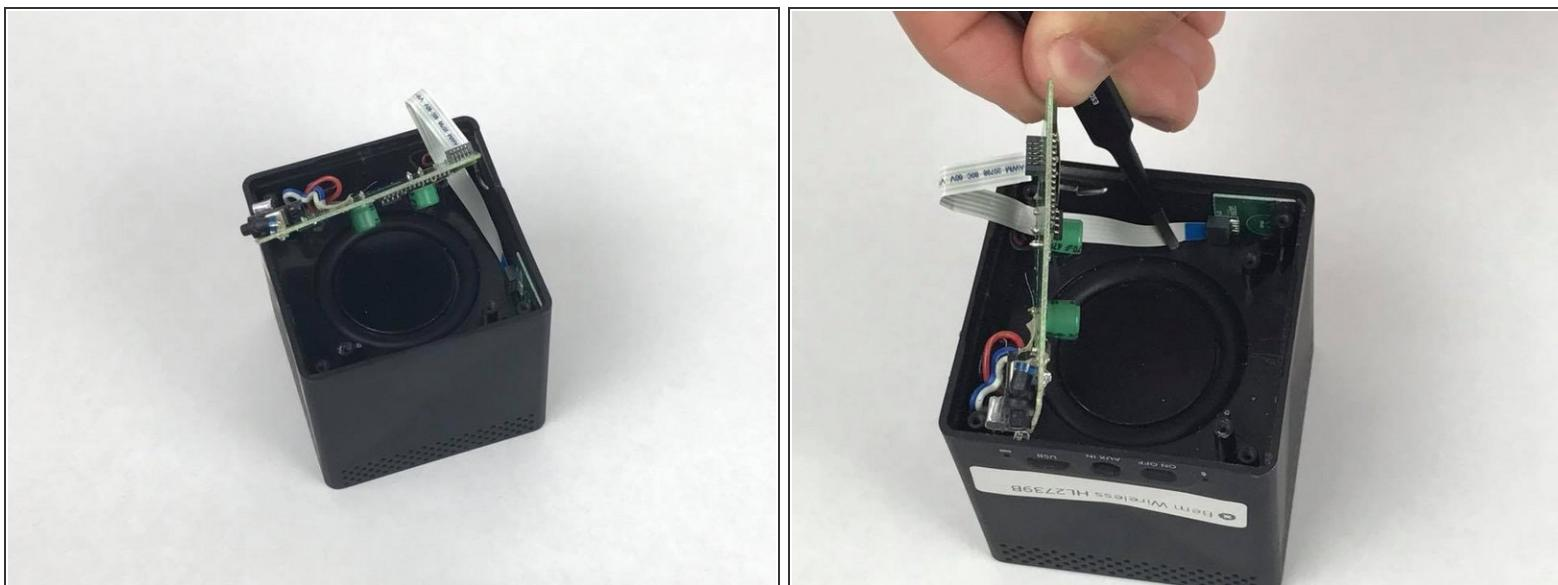
! Gently re-position the motherboard so you can access the bus wire connected to the speaker.
