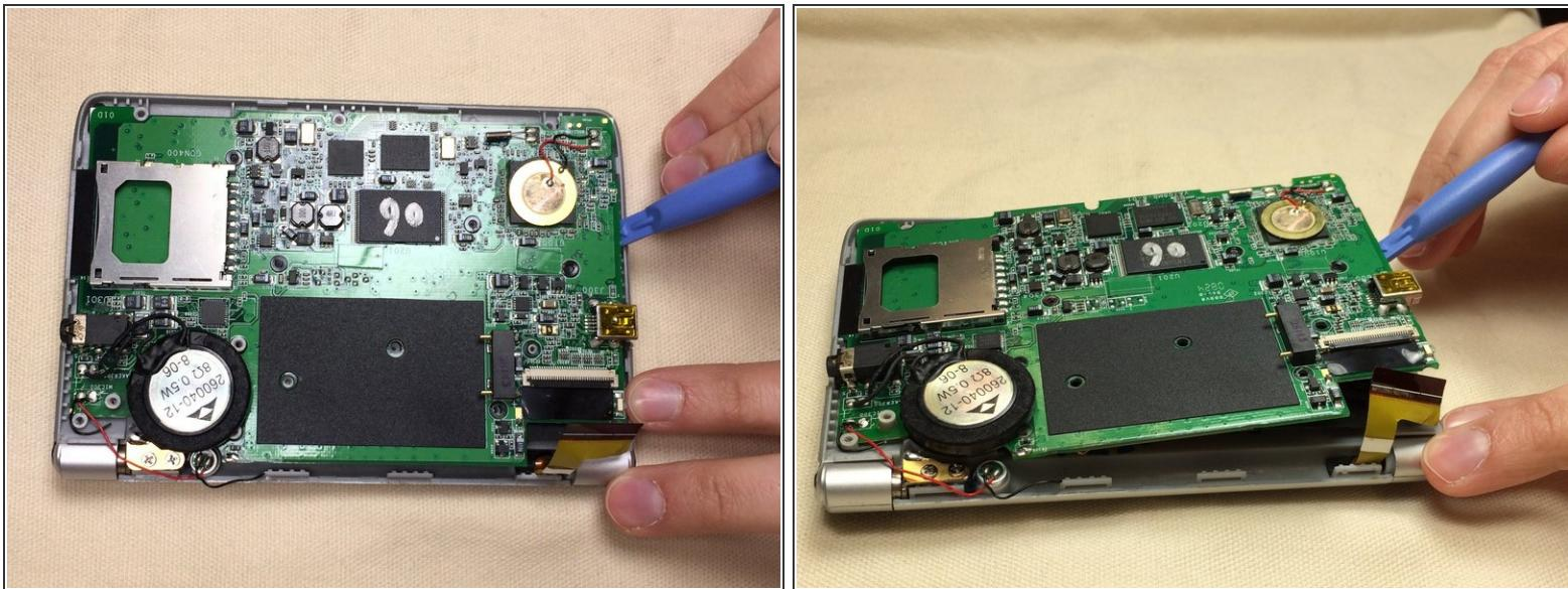
**⚠ WARNING:** All screws must be removed before you begin this step. Do not forcefully pry apart the motherboard with screws still in it because you may damage it.
