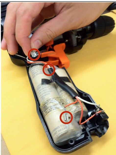
**⚠️ SHOCK WARNING:** Ensure wire ends do NOT touch each other! Disconnect the battery from the drill by pulling out the 3 terminals.
