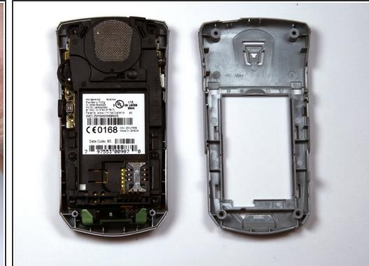
*(i)* The keypad cover may fall out of the housing when prying the housing apart.
