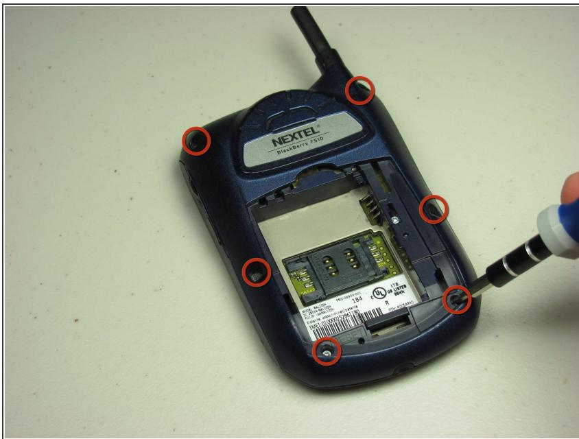
*(i)* Remove the battery cover and battery before continuing.
