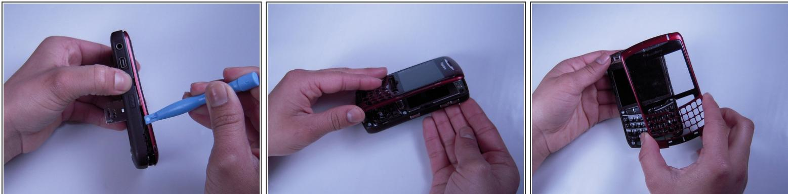
! Be careful not to damage the front cover's plastic clips while trying to separate it from the phone.
