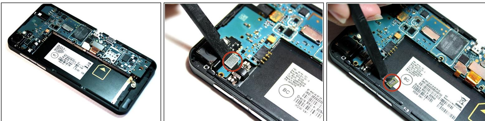
**⚠** Use the nylon spudger, which is a black plastic tool, to avoid any damages on the internal parts of the motherboard.
