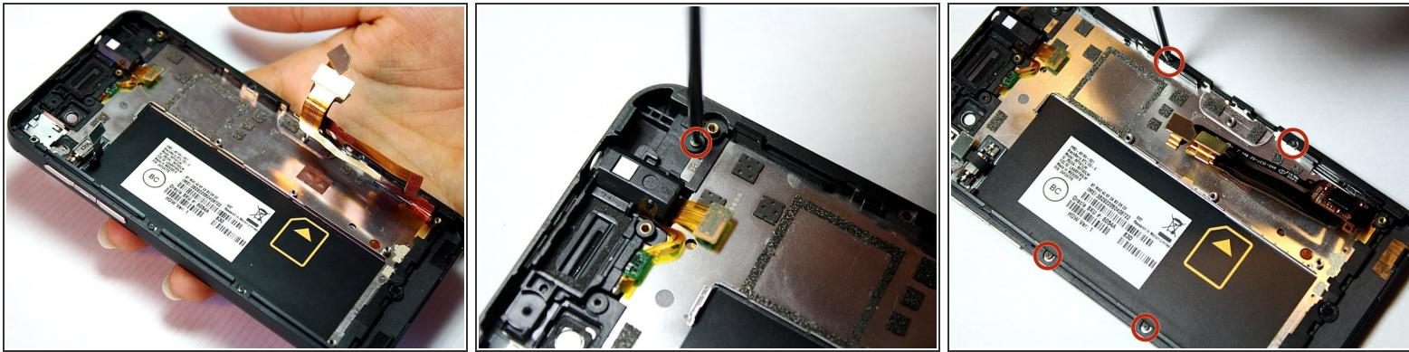
**⚠** The screen is fragile and may crack if the screws are not removed carefully.
