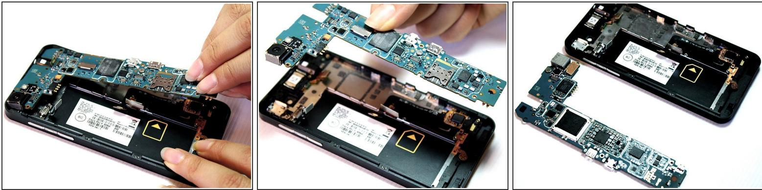
**⚠** The motherboard is fragile. Make sure all connectors have been detached before you remove the motherboard.
