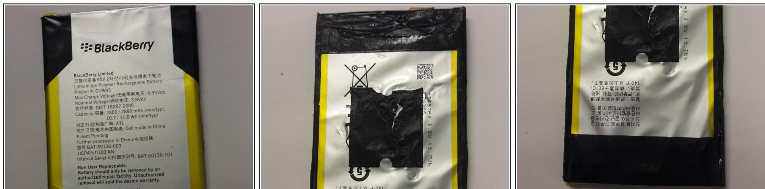
⚠ If this is the original battery, it might be hold down by VERY strong adhesive on the top, middle and bottom part. Be careful not to damage the battery
