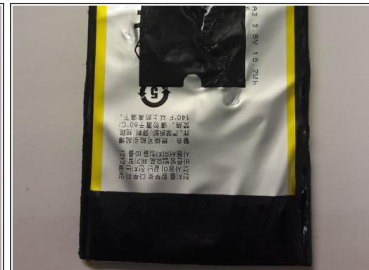
⚠ If this is the original battery, it might be hold down by VERY strong adhesive on the top, middle and bottom part. Be careful not to damage the battery
