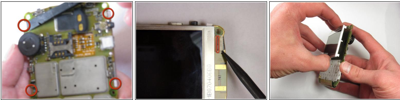
*(i)* The clips disengaged in the next bullet may weaken and break after unclipping them.
