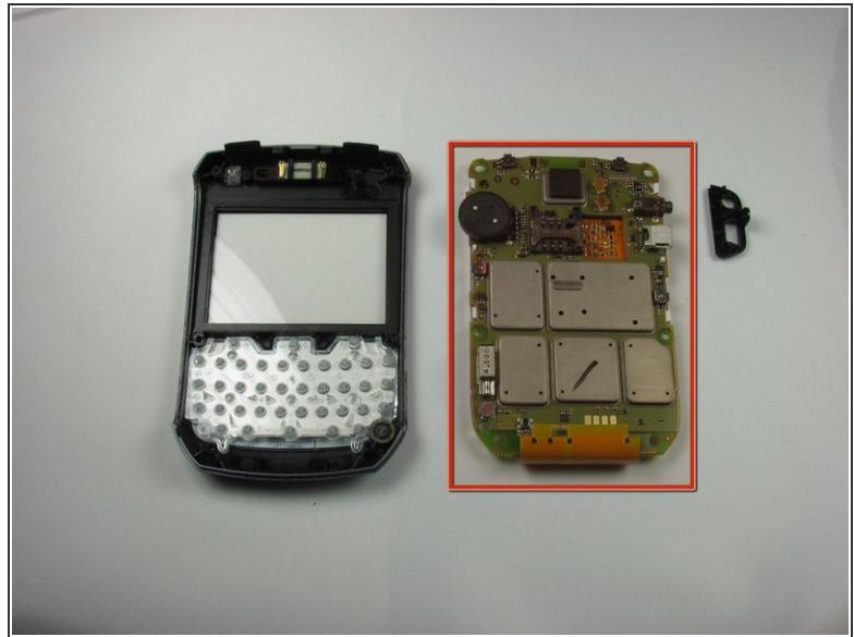
*(i)* The logic board removed in the next bullet is the entire circuit board circled in Picture 2.
