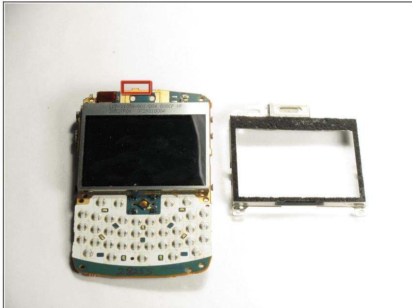
ⓘ Place the motherboard on a flat surface with the LCD screen face up.
