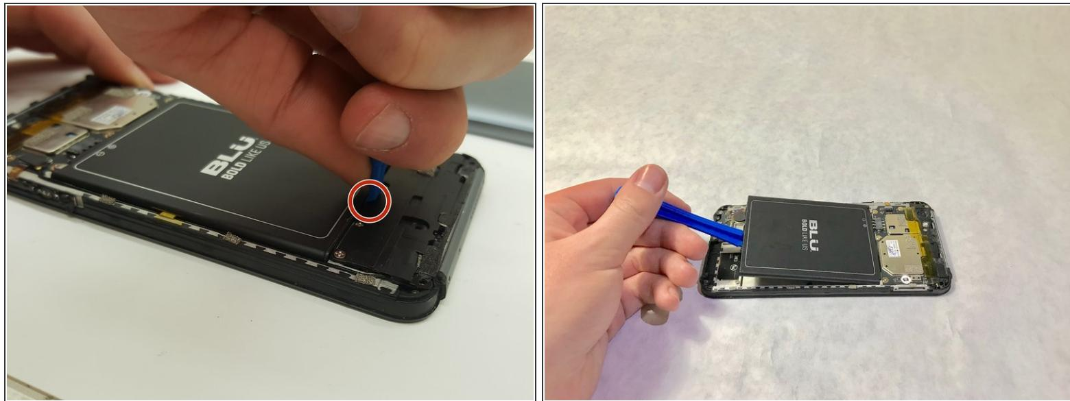
*(i)* There is a patch of adhesive underneath the battery, which can make it difficult to remove.
