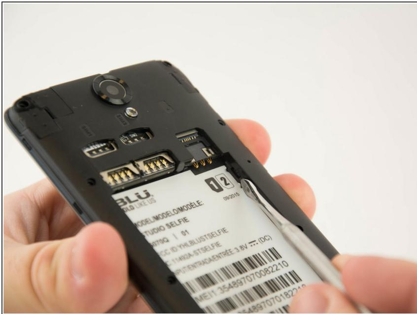
**i** Where the battery rested before, you will find a small clip that holds down the midframe.
