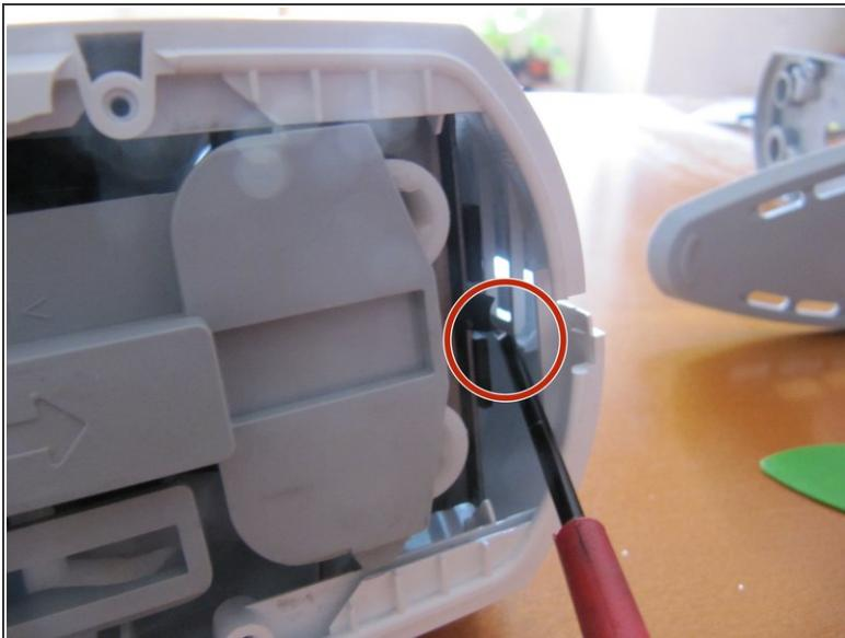
⚠ The first step is somewhat tricky. Use a long screwdriver to release the first part at the top.
