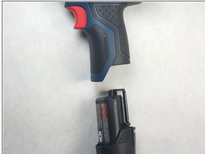
! Remove the battery prior to working on the drill
