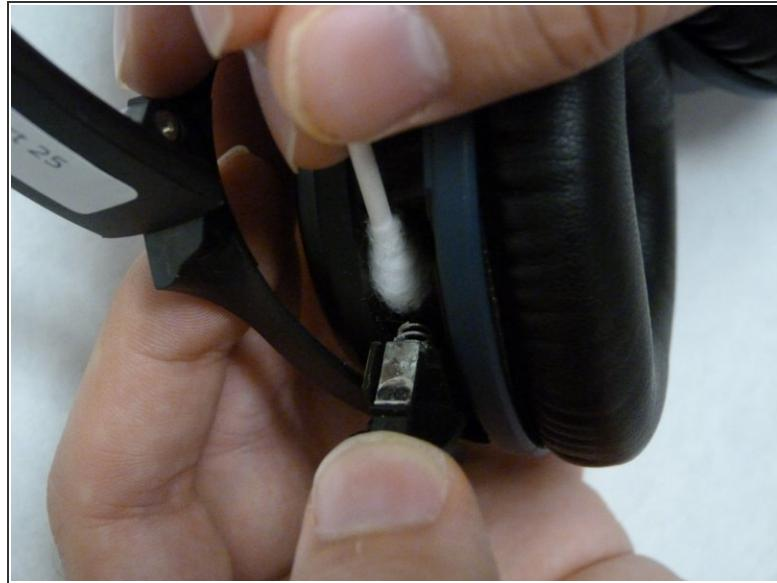
⚠ Do not allow battery corrosion to come into contact with your skin or eyes.
