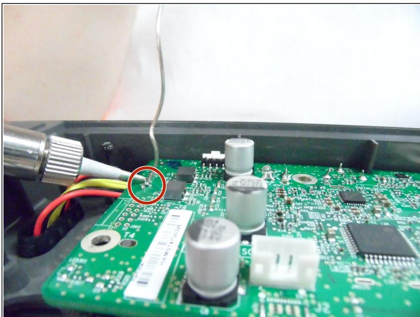
**i** Replace old logic board with the new logic board. Place the wires into the solder holes and solder in place. Reassemble the SoundDock.
