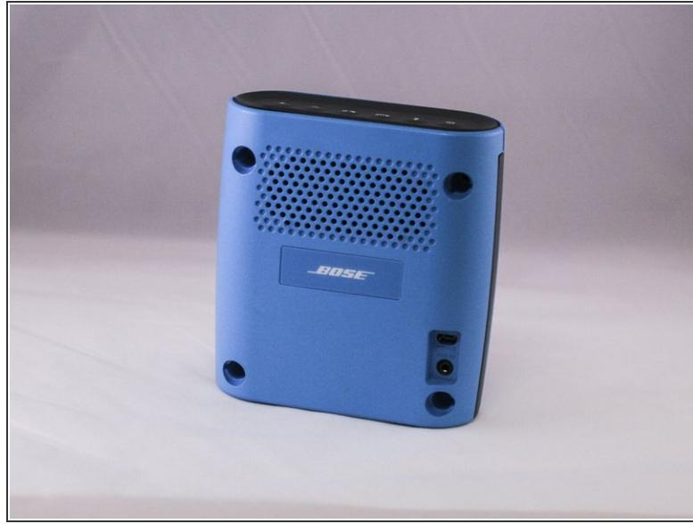
ⓘ Four round, plastic plugs are located on the back of the device.
