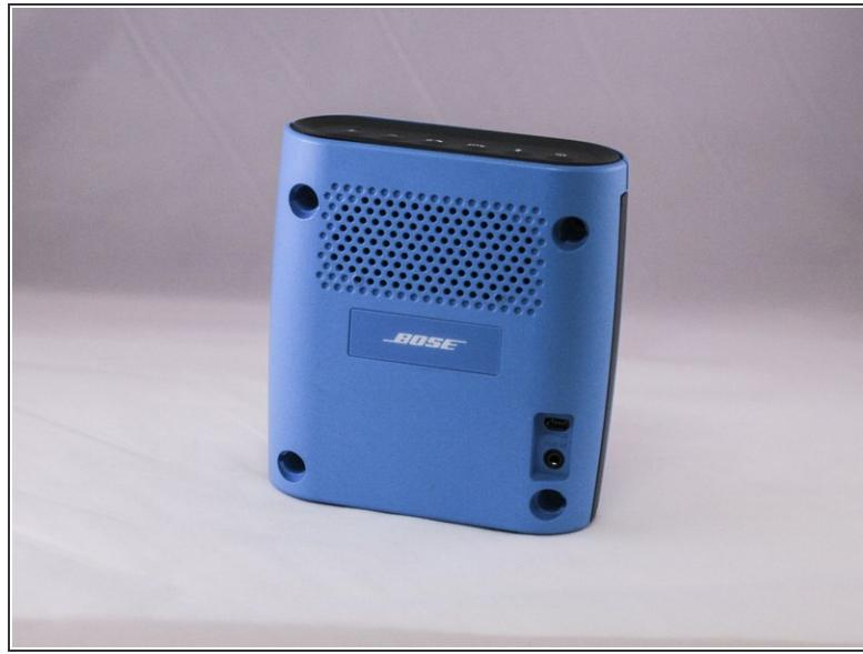
① Four round, plastic plugs are located on the back of the device.
